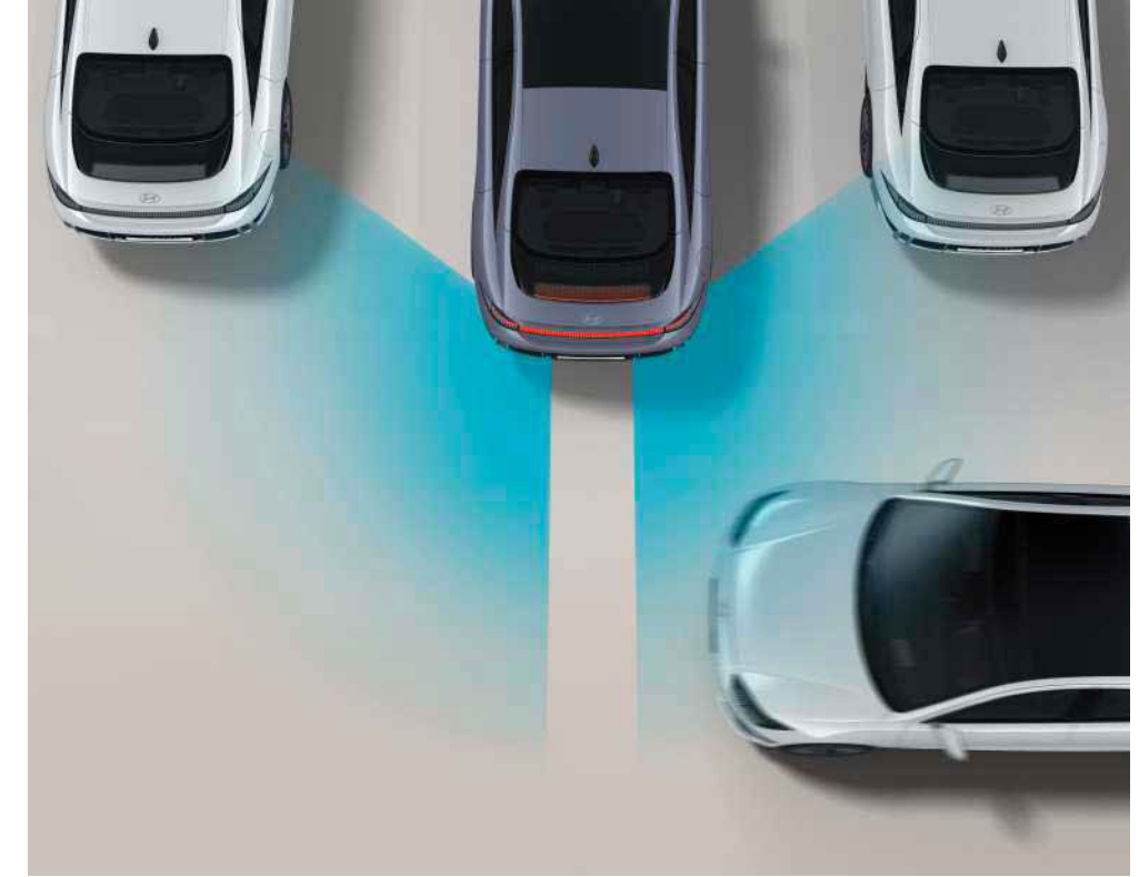
PCA (Parking Collision Avoidance Assist - Reverse)
