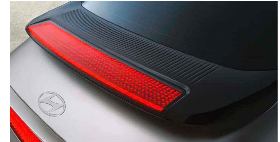
Parametric Pixel High-Mounted Stop Lamp (HMSL)
