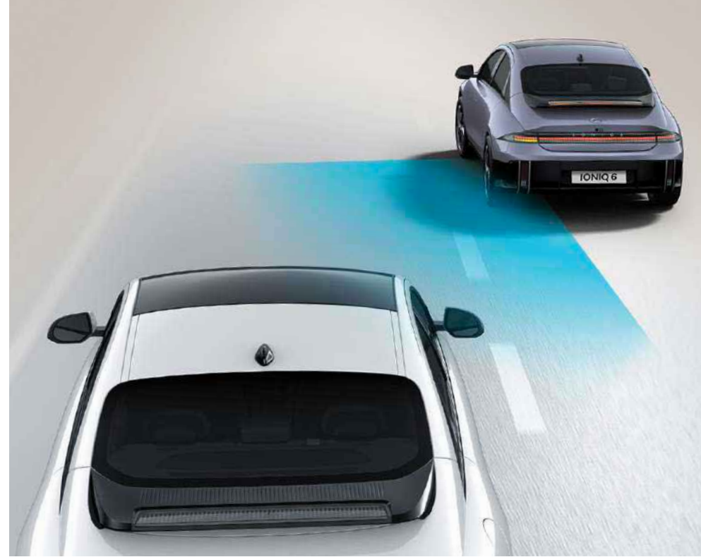
BSVM (Blind Spot View Monitor) & BCA (Blind-Spot Collision Avoidance Assist) - Rear
